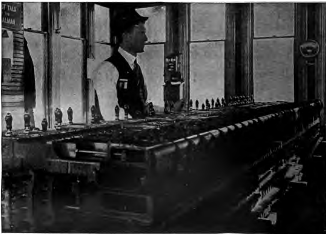
OPERATOR IN THE SIGNAL TOWER. (Showing mechanism by which switches and signals are controlled.)
